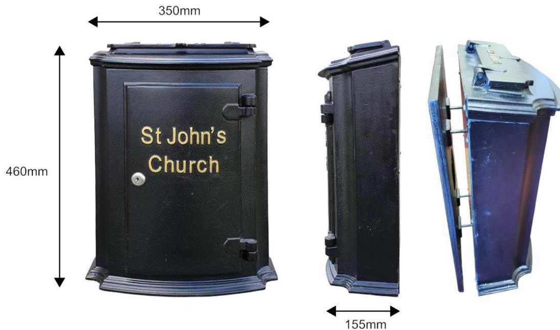
The post box is of a cast iron design and cannot be opened without the key, this ensuring that the mail is secure. It is mounted using a clamp plate shown in the right-hand photograph. The bolts are secured from within the box itself, so that the only way it would be possible to remove the post box is by opening the door with the key.
